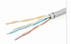
Strip the cable for minimum 75mm, pull the foil or braided shield back over the jacket an wrap the drain wire around the shield.
