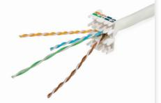
Insert the wires into the cap through the holes.
